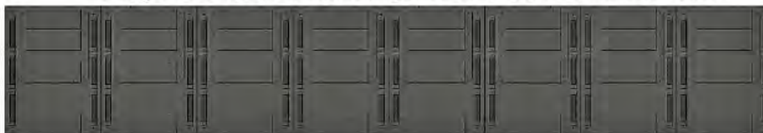
Figure 1: 10 narrow 5kW cabinets and 8 wider 6.25kW cabinets equal the same overall power allocation occupying approximately the same footprint.
