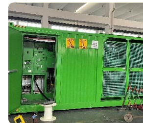
RMU & Tx Container FAT
